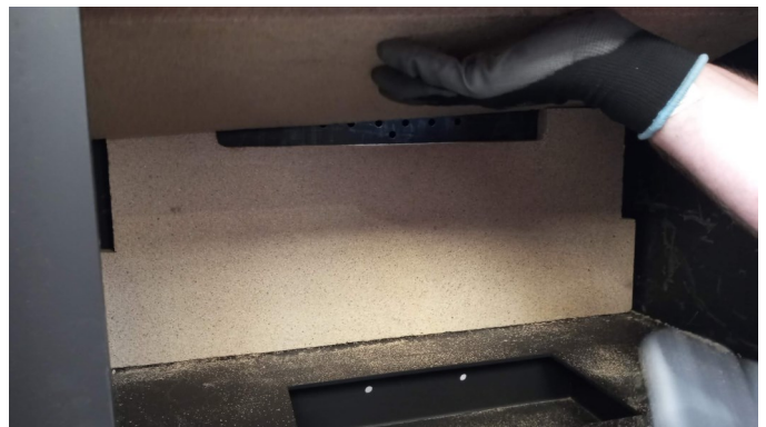
Position the baffles at the bottom of the combustion chamber and remove the upper baffle first and then the lower baffle.
